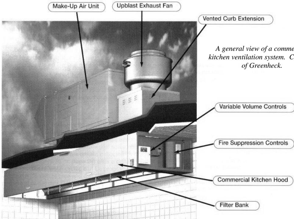
*A general view of a commercial kitchen ventilation system. Courtesy of Greenheck.*
