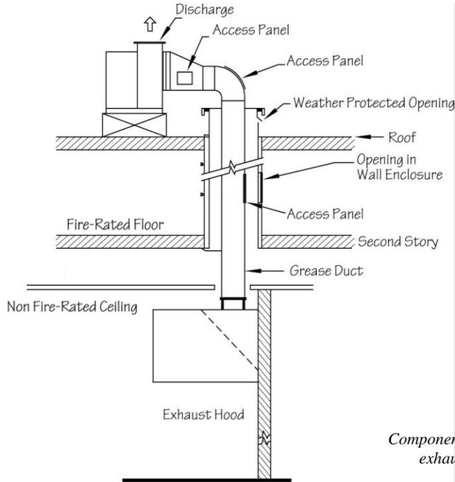
*Components of a typical exhaust system*
