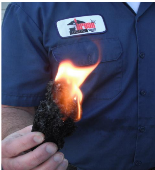
A “chunk” of grease taken out of a restaurant exhaust system, lit with one match
