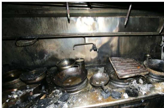
Effects of heat on stainless steel kitchen components: (1) Because stainless steel is designed to resist ferrous corrosion/oxidation, when exposed to high heat stainless steel doesn't show the characteristic "rust" color as readily as do other ferrous materials, and (2) both photos show areas of higher local heat in the "clean burn" patterns, where the metal was too hot for soot to stick to it.
