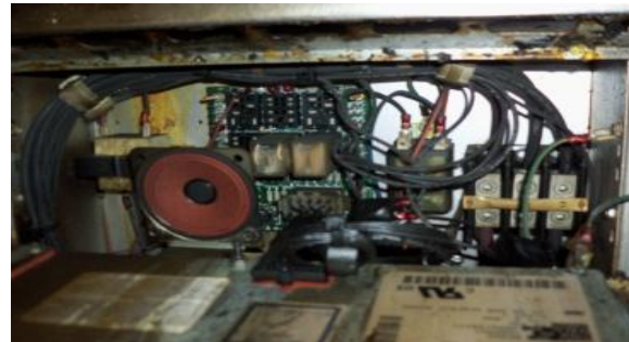
Control bays can be full of grease - fuel to burn - but this non-burnt unit looks clean! For more information on this case see Case Studies Chapter
