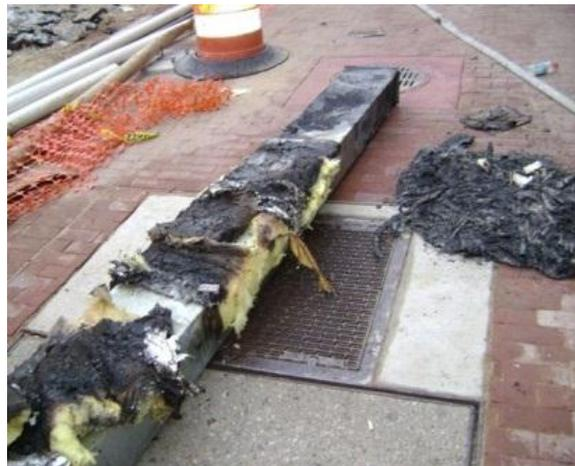
*Exterior of the removed duct previously covered with insulation*
