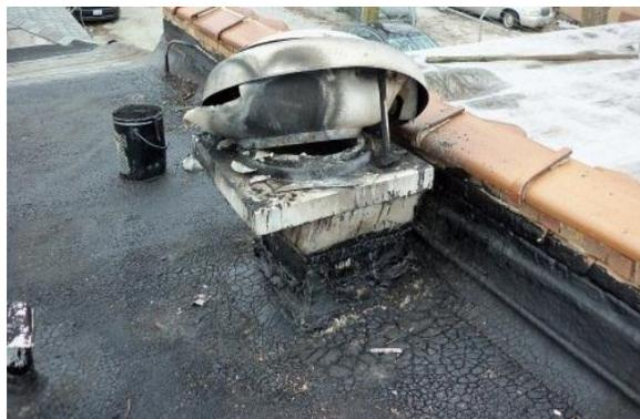
*Residue of an aluminum upblast fan after a fire*
